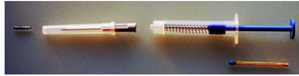
Fig. 2. RFID chip, injection system.
